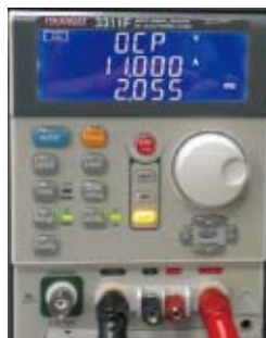
Figure 14 3311F with BMS for over current discharge test result ( continuous STEP pulse )
