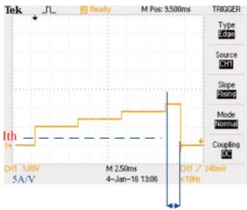
over current protection time is about 2.056ms
