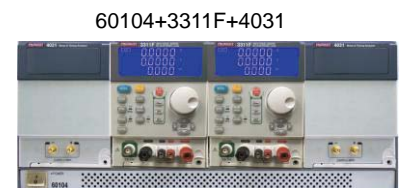
60104 is the mainframe for modules
