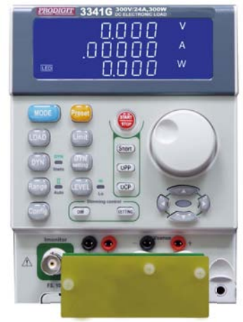
Short test fixture is installed on load input by plug-In operation
